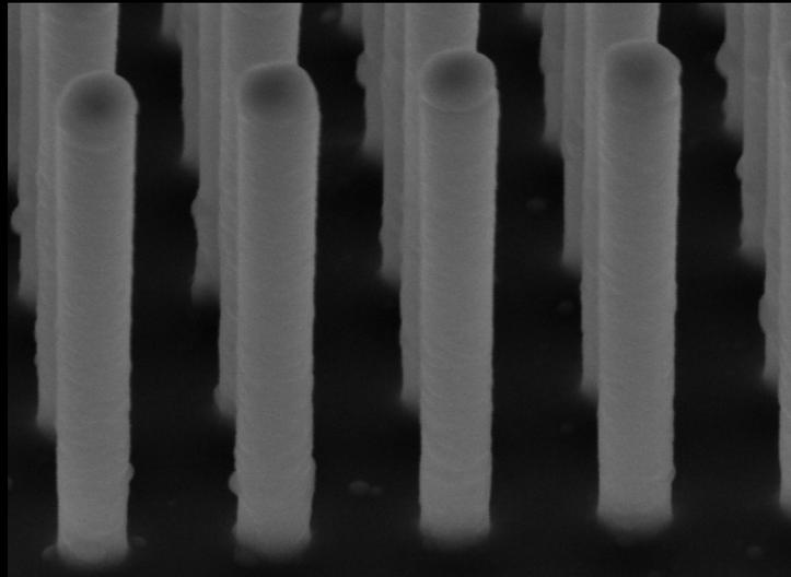
**Si NWs with Si<sub>x</sub>N<sub>y</sub> coating**
